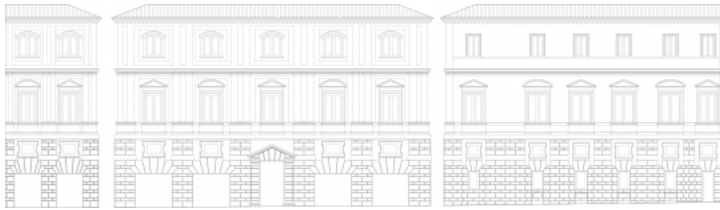
Fig. 19b. Palazzo Stati Maccarani, elevations: (top) existing condition; (bottom) hypothetical reconstruction of original condition. Representation by author.
