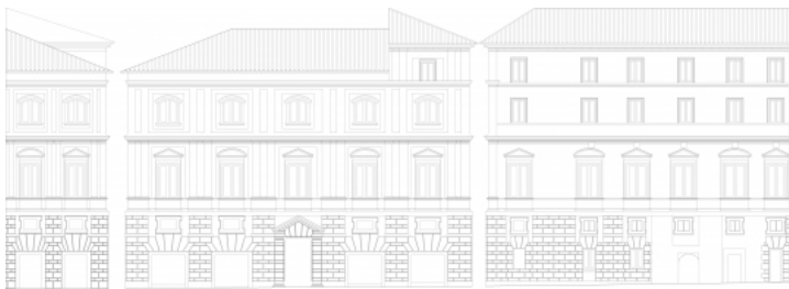
Fig. 19a. Palazzo Stati Maccarani, elevations: (top) existing condition; (bottom) hypothetical reconstruction of original condition. Representation by author.
